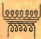
STEP - UP TRANSFORMER.
