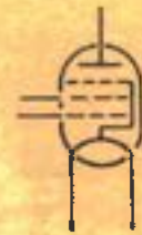
5 ELECTRODE VALVE (PENTODE).
