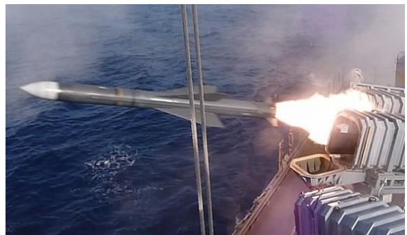
Figs 46 & 47 MM-38 Exocet missiles within canisters and launching.
