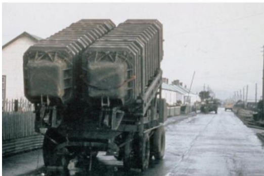
Figs 46 & 47 MM-38 Exocet missiles within canisters and launching.
