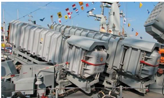
Figs 46 & 47 MM-38 Exocet missiles within canisters and launching.
